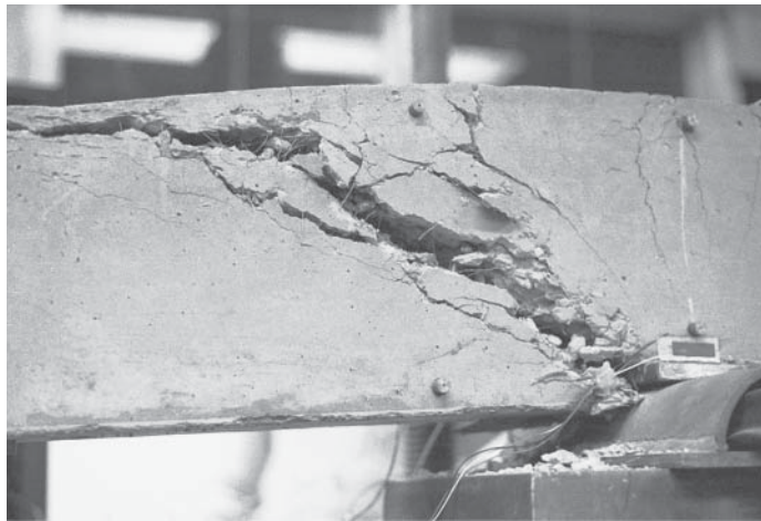
Shear failure near a middle support.
