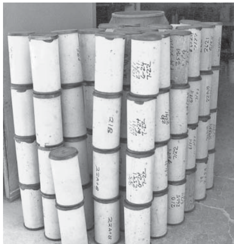
Standard capped cylinders ready for testing.
