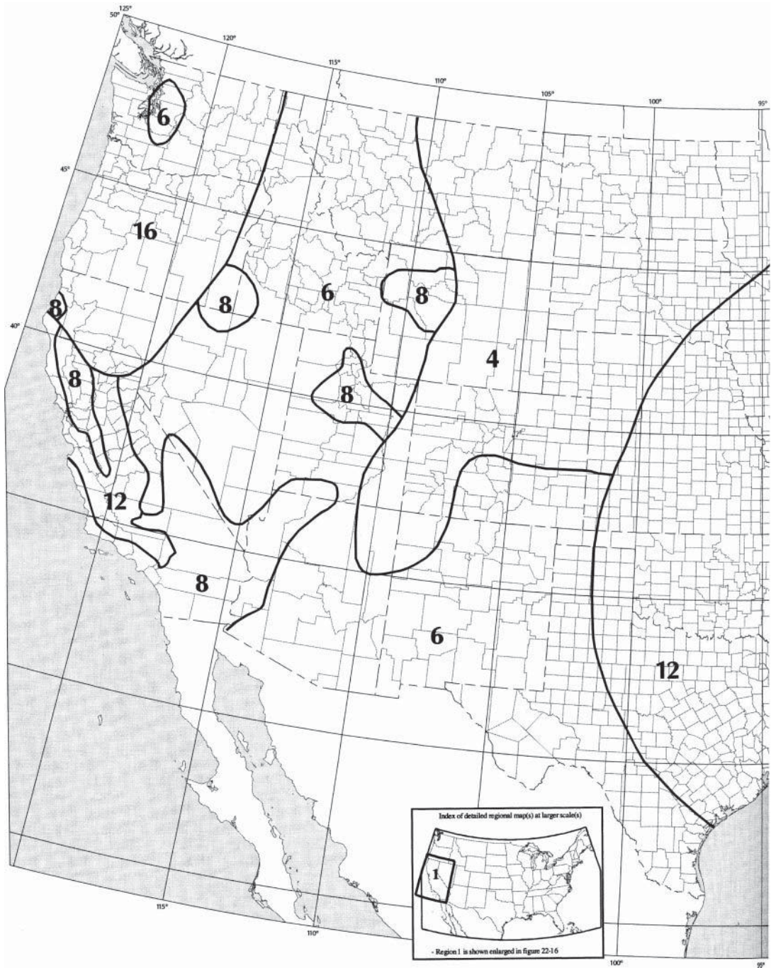
Figure 20.2a Long-period transition period, T_L (sec), for the conterminous United States. ASCE 7-10 Minimum Design Loads for Buildings and Other Structures, 2010. With permission from ASCE
