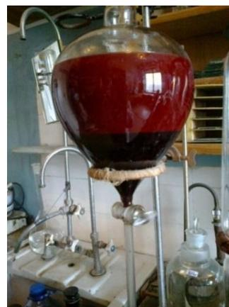
**c) Process of liquid – liquid extraction
