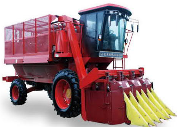
9-rasm. 4M3A rusumli paxta terish mashinasi va modul tayyorlagich
