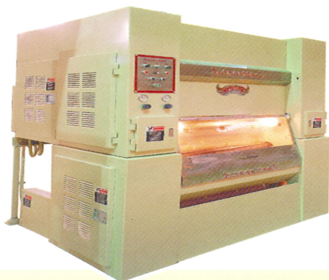
4-rasm. “Fenniks Rotobar” g‘o‘lali jinining tashqi ko‘rinishi.
