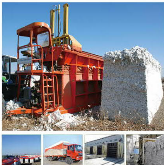
9-rasm. 4M3A rusumli paxta terish mashinasi va modul tayyorlagich
