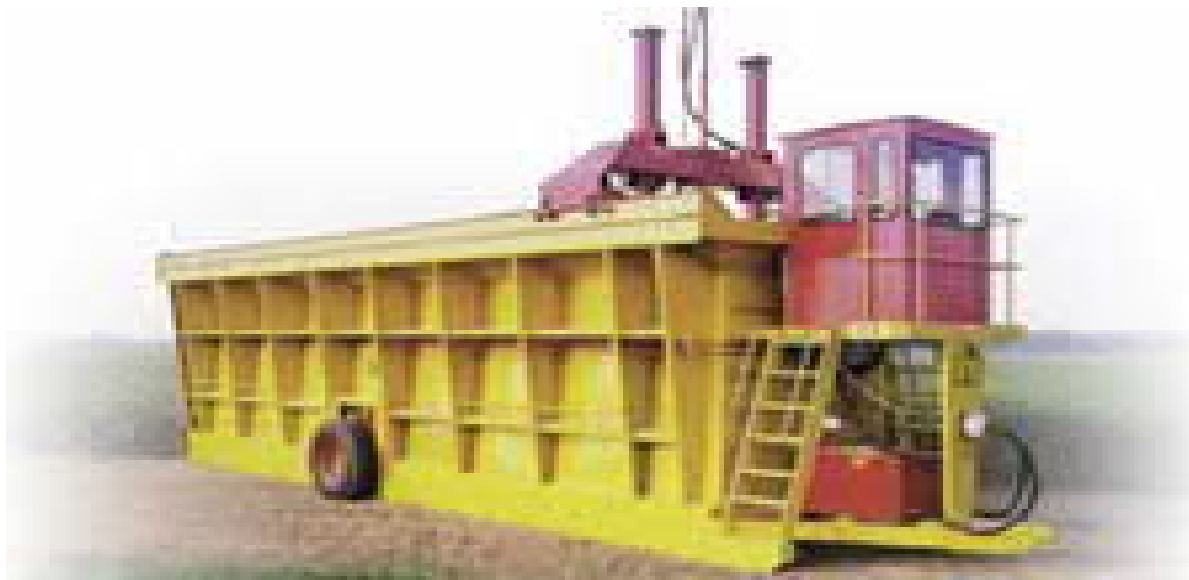
10-rasm. Paxta moduli tayyorlagichi
