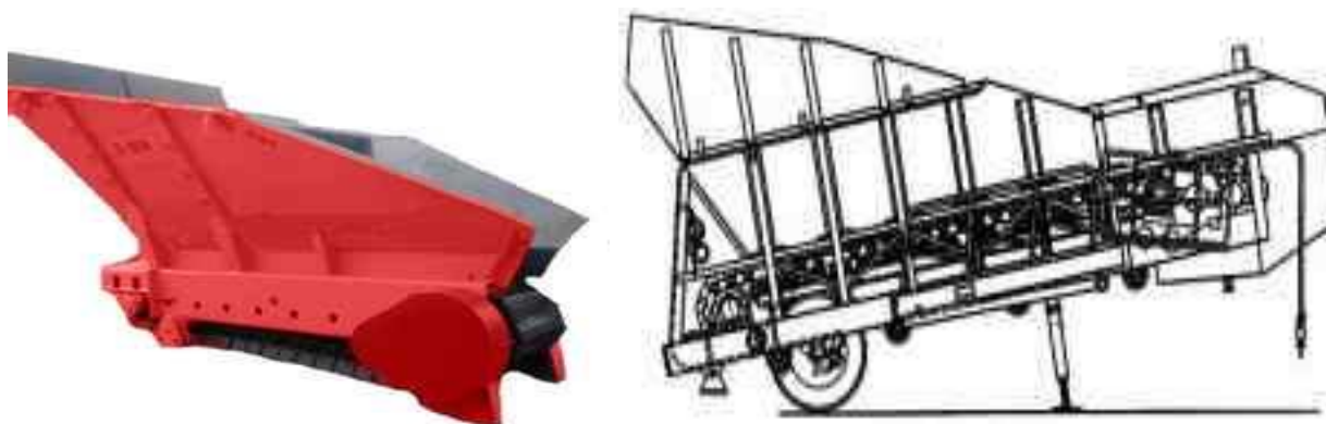
28–rasm. Zamonaviy TK-16 rusumli siljiydigan plastinkali bunker-ta'minlagich.
