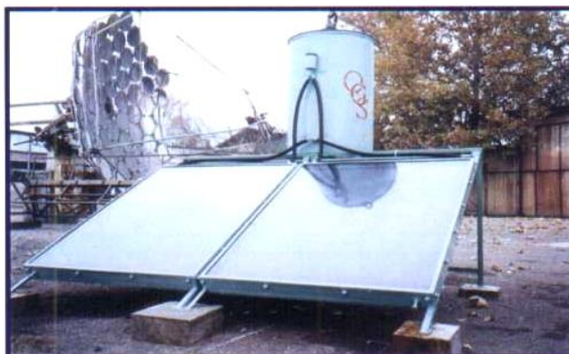
1.2.13-rasm. Quyosh isitgichining sathi 4 \text{ m}^2 va issiq suv jamlovchi bakining hajmi 300 l bo‘lgan 2 konturli suv isitgich qurilma
