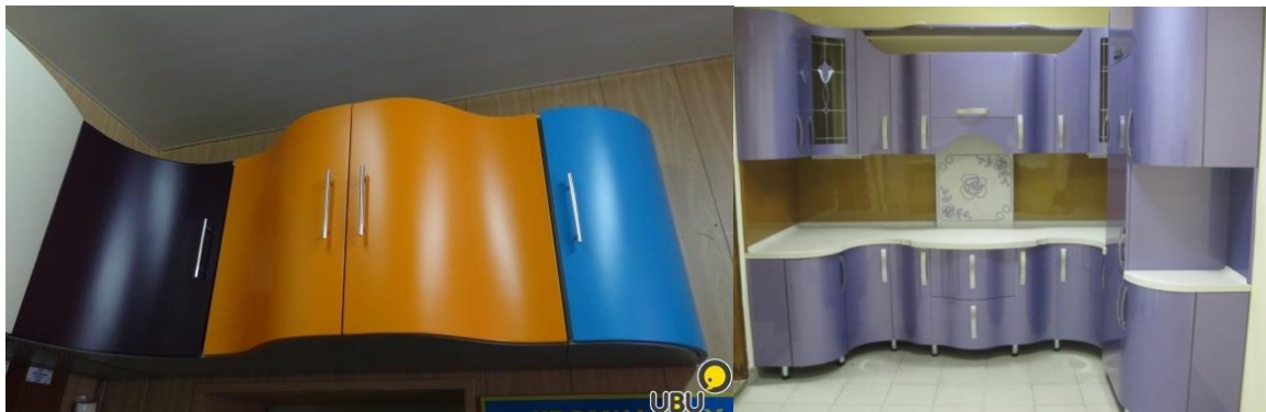
5.8-rasm. Egib yelimplash usulida yasalgan mebel detallari
