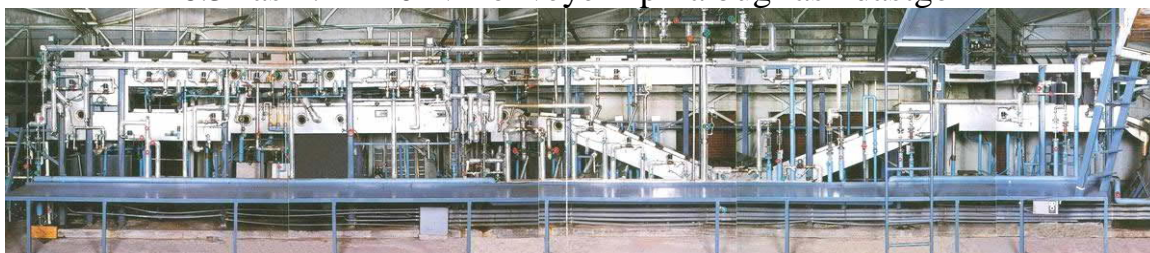
6.3-rasm. FY201V konveyerli pilla bug'lash dastgohi
