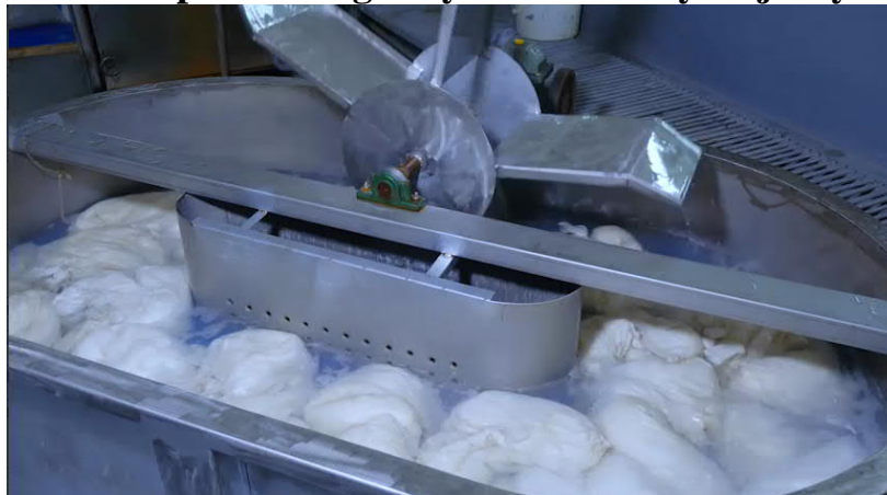
5.6-rasm. Ipak momig'ini yuvish va chayish jarayoni
