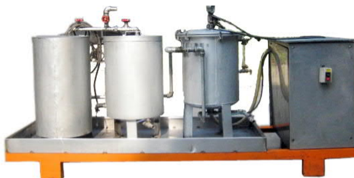
6.3-rasm. FY201V konveyerli pilla bug'lash dastgohi
