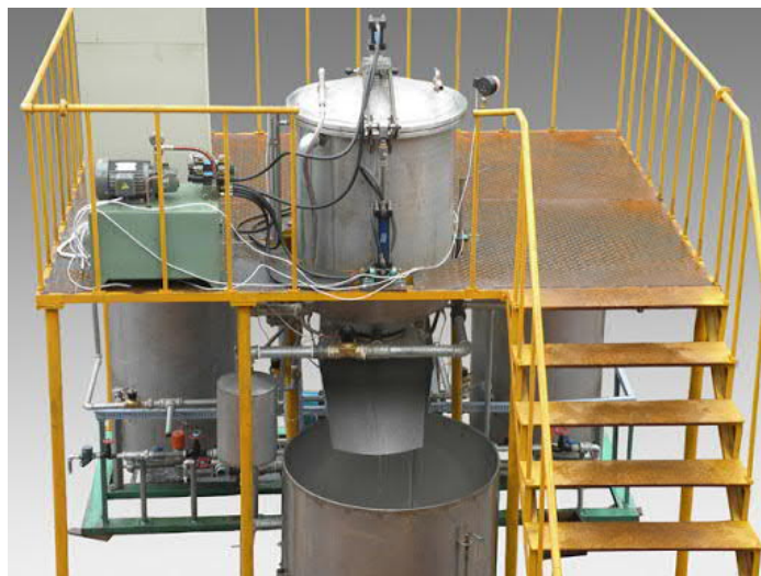
4.8-rasm. Zamonaviy pillani ichiga vacuum oraqli suv to'ldirish dastgohi
