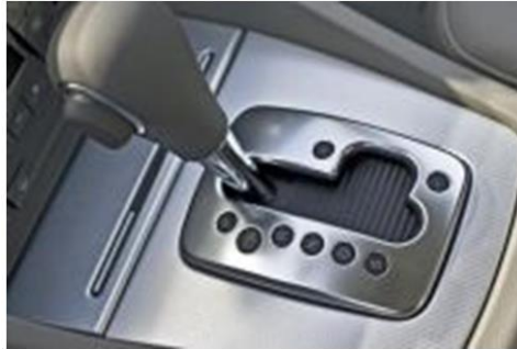
5-rasm. Tiptronik funksiyali AUQni boshqarish richagi
