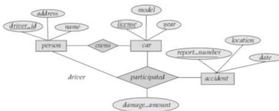
Figure 6.1 E-R diagram for a car insurance company.
