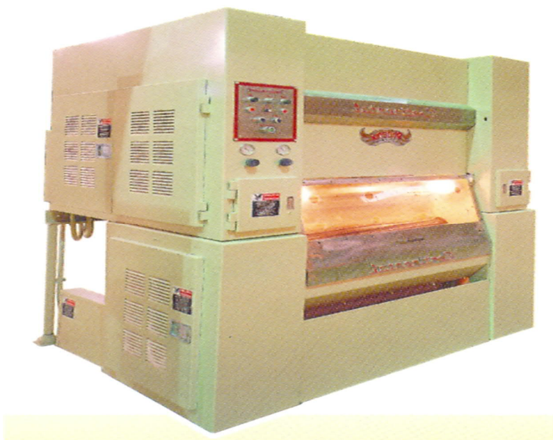
15-rasm. “Fenniks Rotobar” g‘o‘lali jinining tashqi ko‘rinishi.
