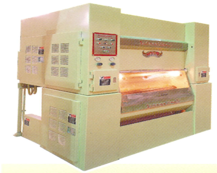
4-rasm. “Fenniks Rotobar” g’o’lali jinining tashqi ko‘rinishi.
