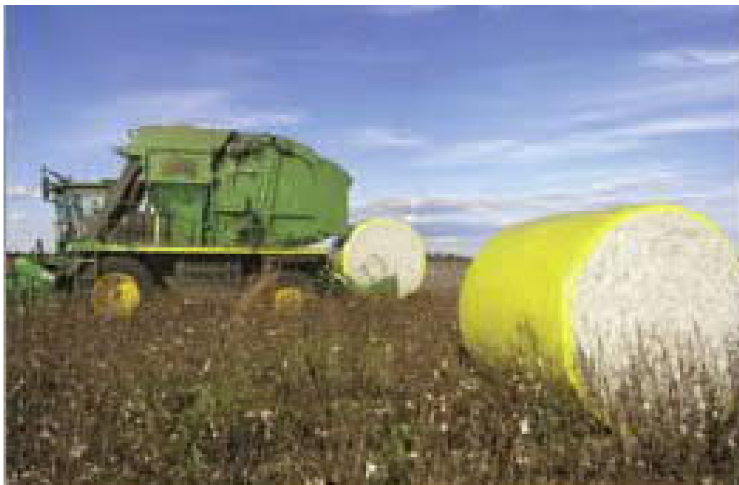
8-rasm. CP690 rusumli paxta terish kombayini va undan paxtani modul chiqarish jarayoni
