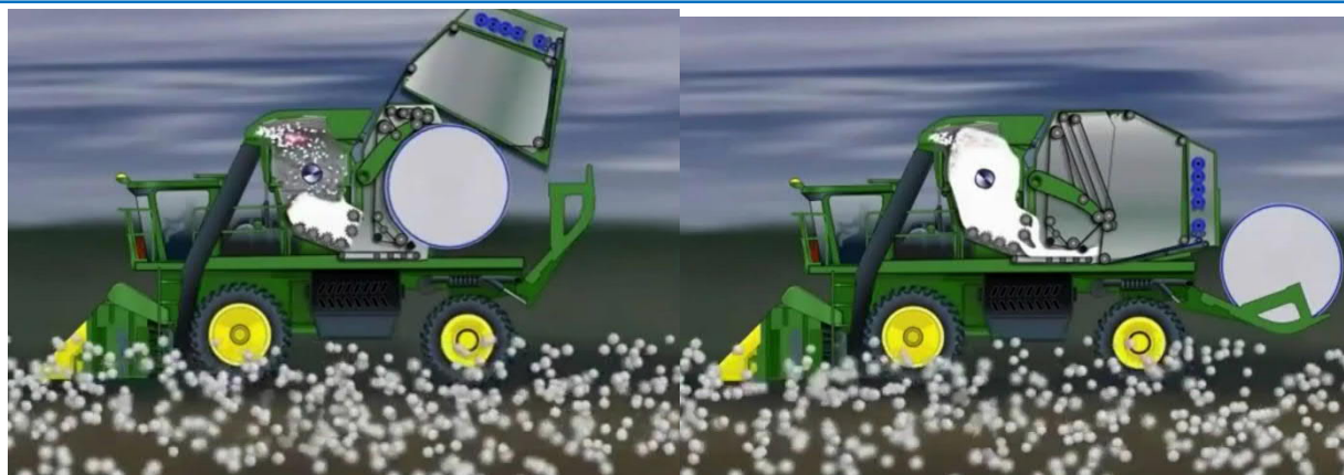
5-rasm. Mashina kombaynida tayyorlangan paxta modulini chiqarish jarayoni
