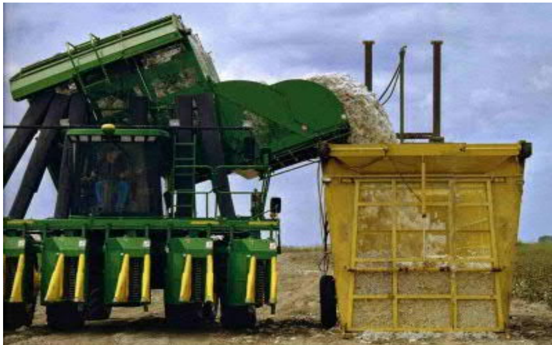
7-rasm. Paxta terish kombayni va undan paxtani modul tayyorlagichga yuklash jarayoni
