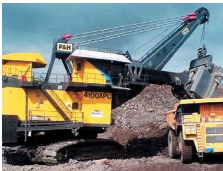
Ris. 6. P&H kompanisining tishli reykali kuch berish tiimli 4100XRS eng katta karyer mexanik ekskavatori.
