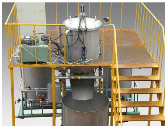
4.8-rasm. Zamonaviy pillani ichiga vacuum oraqli suv to'ldirish dastgohi
