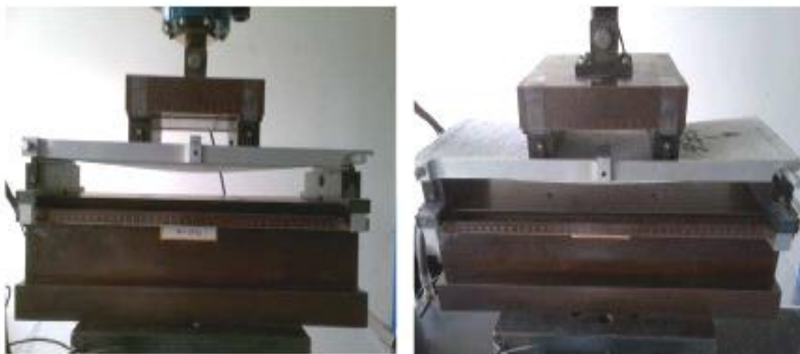
Figure 8: Four bending test. Example of deflection observed with sprayed Ductaf® mixes at 28d
