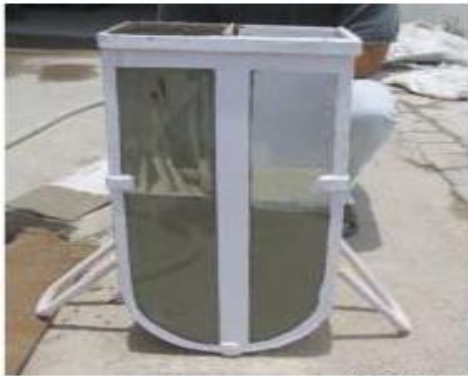
Concrete passing through U-Box Courtesy : Hindustan Construction Company
