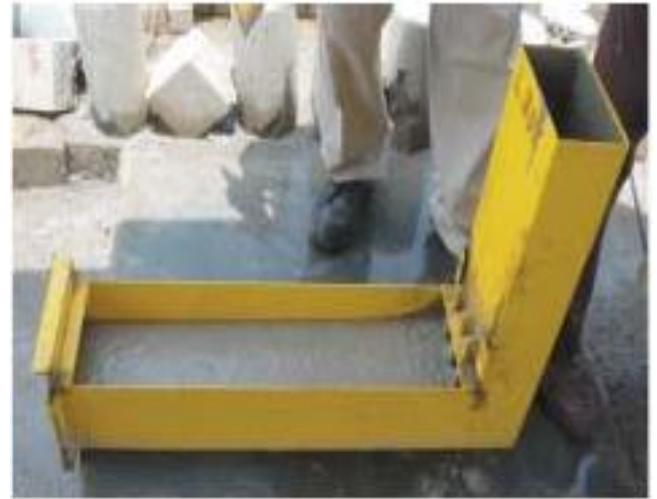
Concrete flowing through L-Box Courtesy : Hindustan Construction Company
