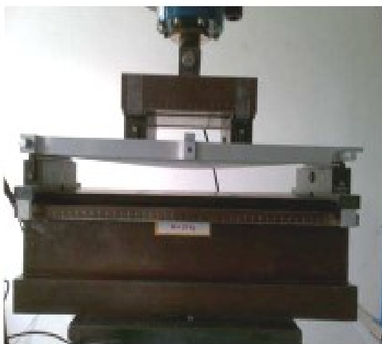
Figure 8: Four bending test. Example of deflection observed with sprayed Ductal® mixes at 28d
