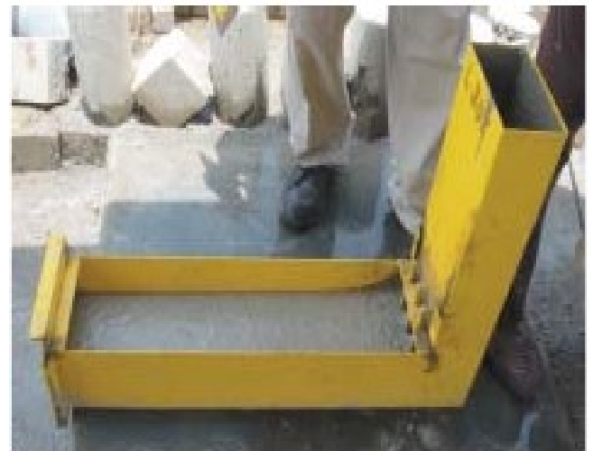
Concrete flowing through L-Box Courtesy : Hindustan Construction Company
