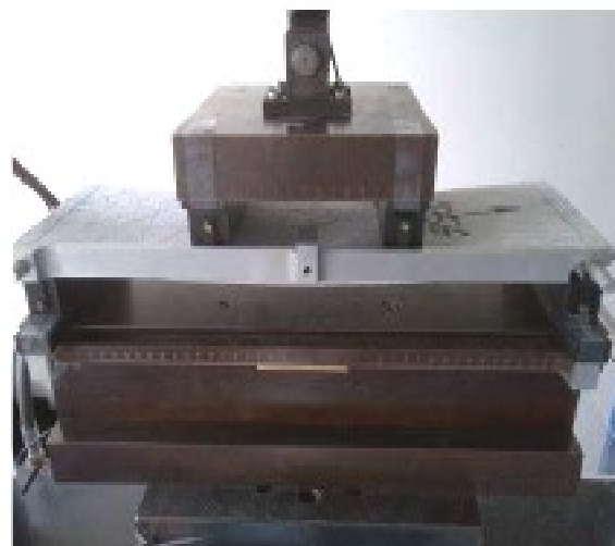
Figure 8: Four bending test. Example of deflection observed with sprayed Ductal® mixes at 28d
