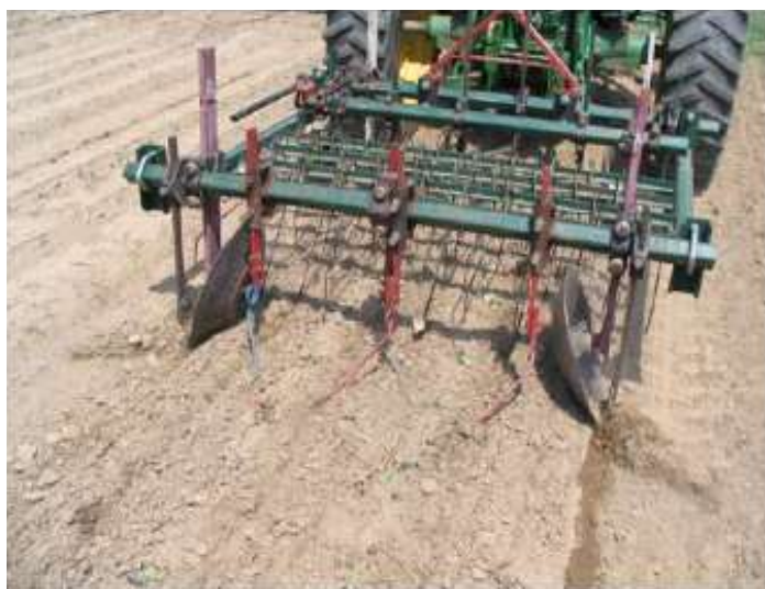
Figure 5. Flex-tine weeder with torsion rods
