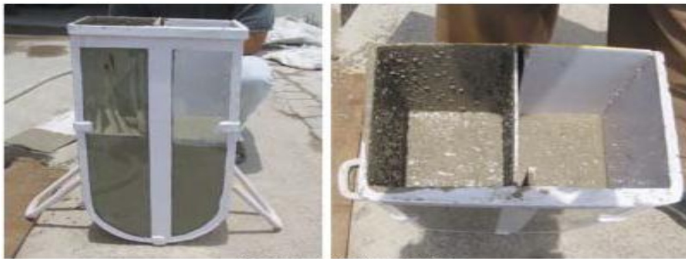
Concrete passing through U-Box Courtesy : Hindustan Construction Company
