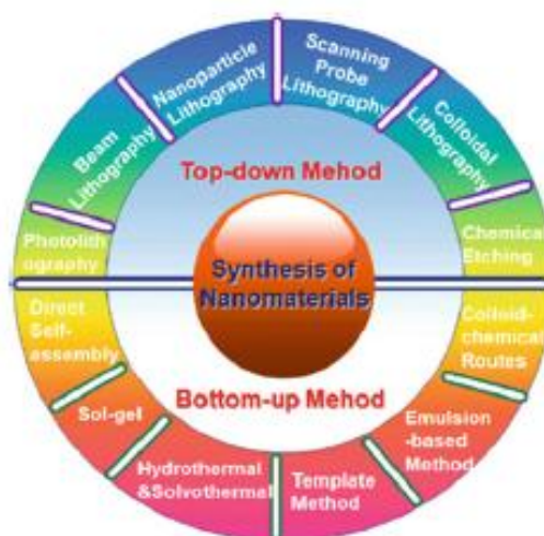
Fig. 2.8 Schematic illustrations of the synthesis methods of nanomaterials (Qiao et al. 2011)
