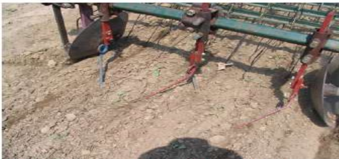
Figure 9. Torsion weeder—two pairs of torsion rods adjusted for twin row cabbage
