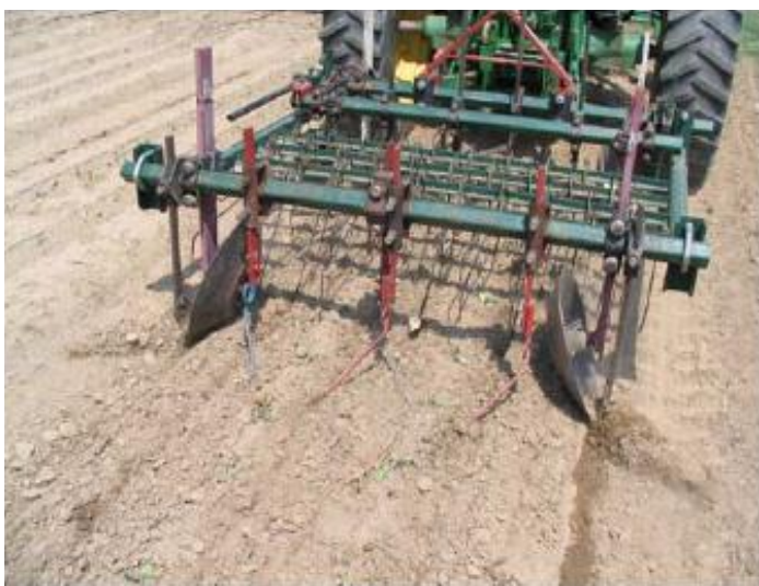
Figure 5. Flex-tine weeder with torsion rods
