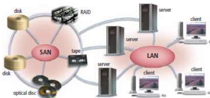
Figure 14-28b (a SAN provides centralized storage for servers and networks)
