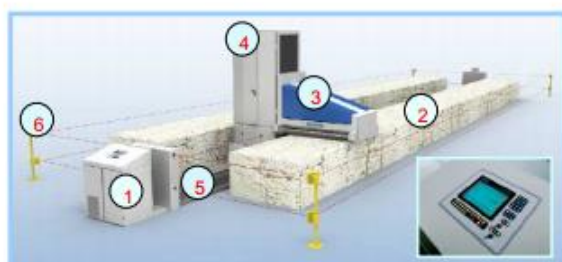
(1) Control unit, (2) fiber bales, (3) working head with tooth discs, (4) Swivel tower, (5) air duct for material transport, And, (6) protective light barrier.
