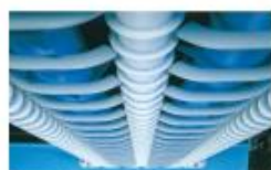
Production in distributed air flow spinning mode. Using impinging jet air generation in radial holes of the rotor.
