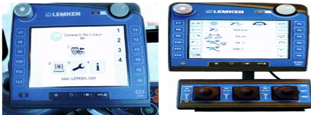
3.5-rasm. Belgilar va piktogramma qurilmasi (a) va plugni boshqarish uchun djoystli SSIISOBUS terminali (v)
