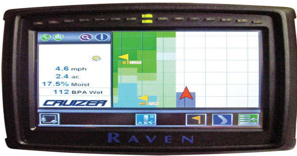
19-rasm. Raven firmasining hosildorlikni oniy aniqlash tizimi monitori
