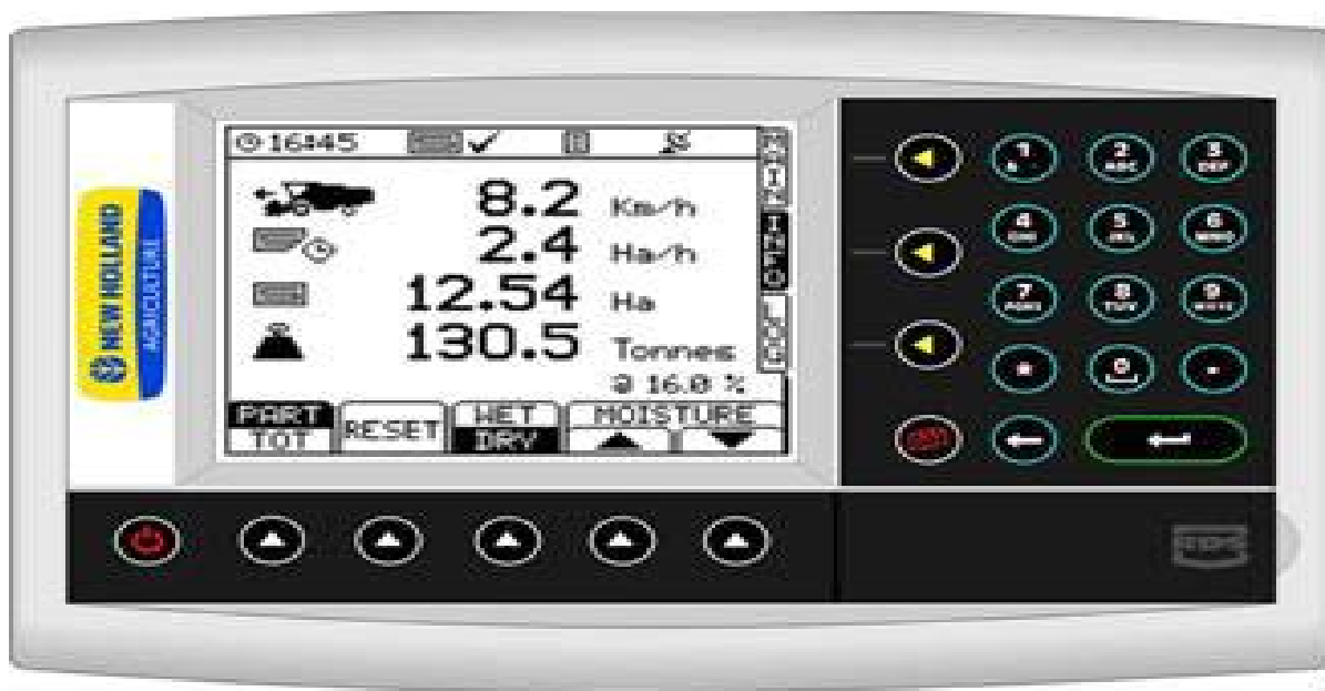
17-rasm. New Holland kombaynlarining hosildorlikni lahzalarda aniqlash tizimining monitori
