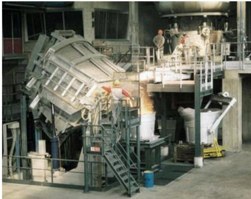
1.7-rasm. Tigelli erituvchi induksion pechida po‘lat eritish jarayoni
