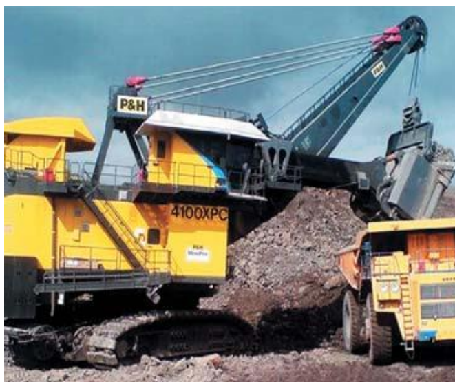
5-rasm. P&H kompanisining tishli reykali kuch berish tiimli 4100XRS eng katta karyer mexanik ekskavatori
