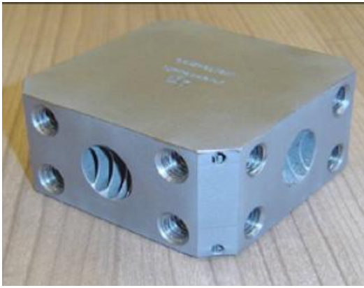
Murakkab ichki kanallarga ega gidravlik prototip, (Manba: EU project COMPOLIGHT)
