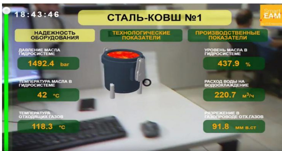
1.5-rasm. AR-ni INTERPIPE STEEL-da IT-Enterprise-ning SmartEAM yechimida qoʻllash misol
