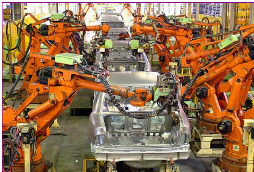
1.3-rasm. Avtomobil organlarining ommaviy-ishlab chiqarish liniyasi Manba: Ford Motor Company.
