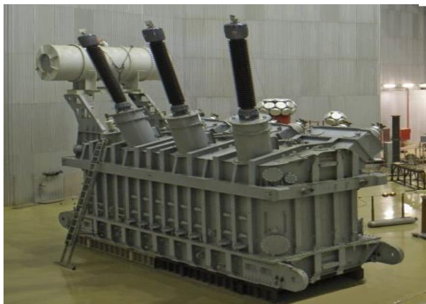
1 – rasm. TIQ-630000/330 tipli kuch transformatori zovodning tajriba zalida
