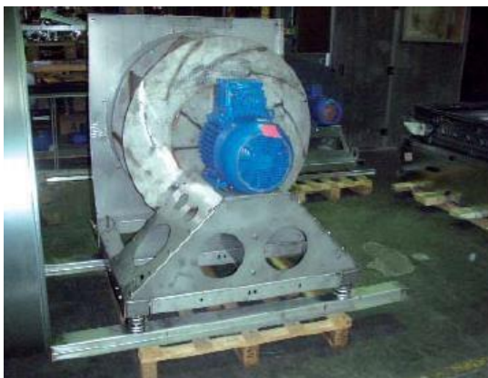
3.27-rasm. Ventilyator – bo‘sh g‘ildirak d = 250...1250 mm
