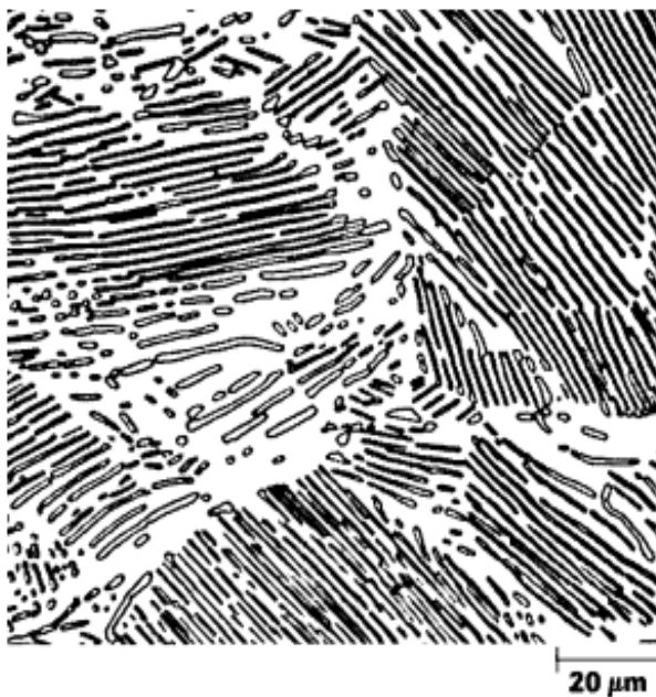
Figure 9.27 Photomicrograph of a eutectoid steel showing the pearlite microstructure consisting of alternating layers of \alpha ferrite (the light phase) and Fe_3C (thin layers most of which appear dark). 500 \times . (Reproduced with permission from Metals Handbook , 9th edition, Vol. 9, Metallography and Microstructures , American Society for Metals, Materials Park, OH, 1985.)
