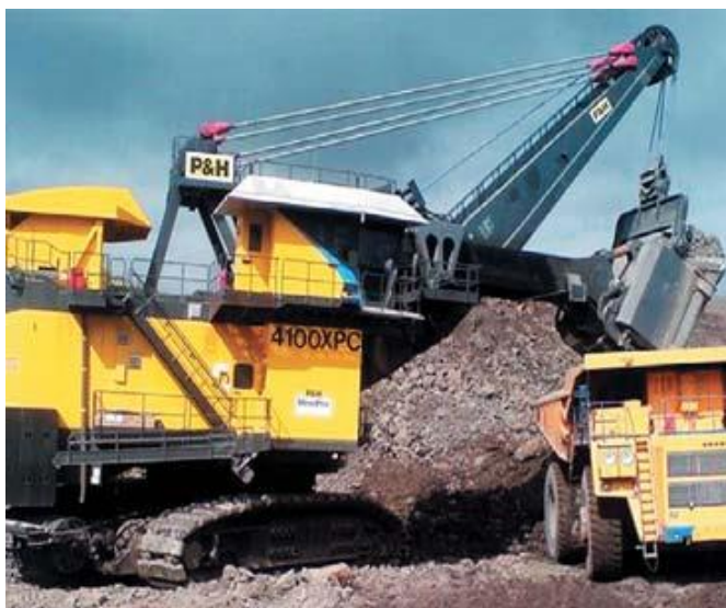
5-rasm. P&H kompanisining tishli reykali kuch berish tiimli 4100XRS eng katta karyer mexanik ekskavatori
