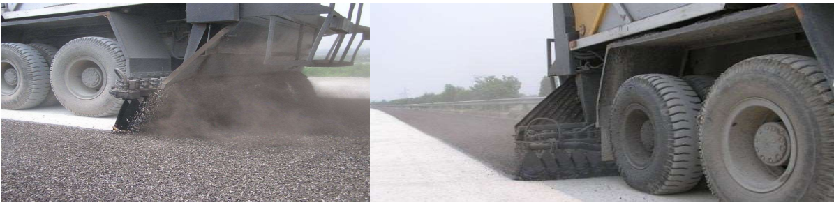
2.33-rasm. DAGANG SX5255TBS chipsilerida sirtga ishlov berish jarayoni
