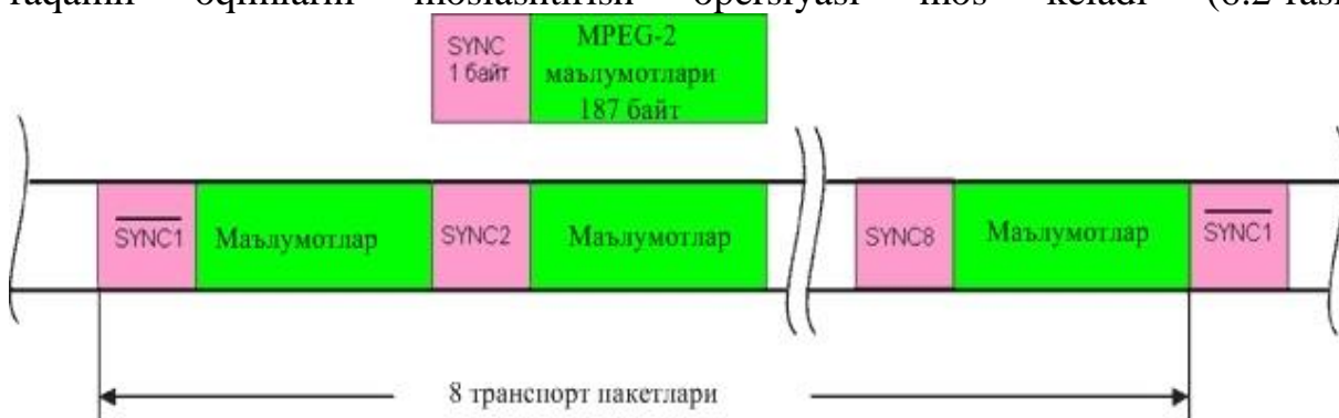
3.5-rasm. MPEG-2 ning transport paketlarining moslashuvi.
