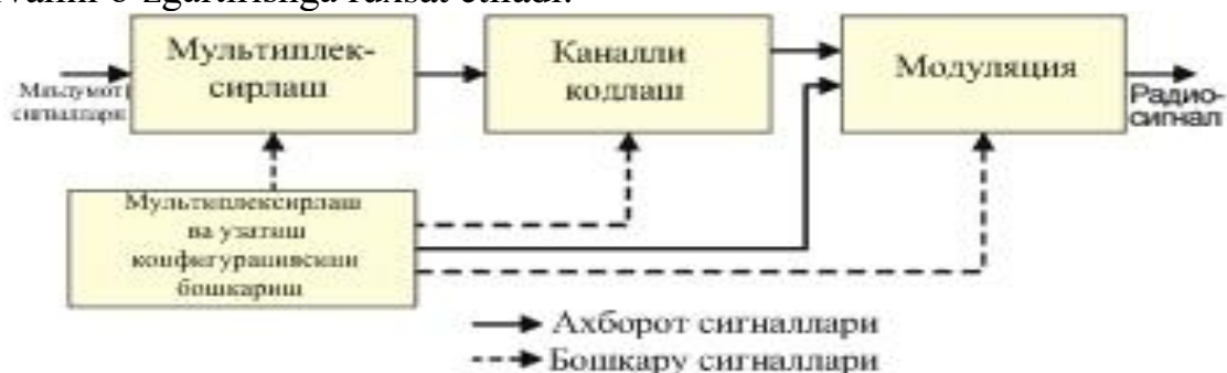
4.18 – rasm. ISDB – T tizimning uzatish chizmasi
