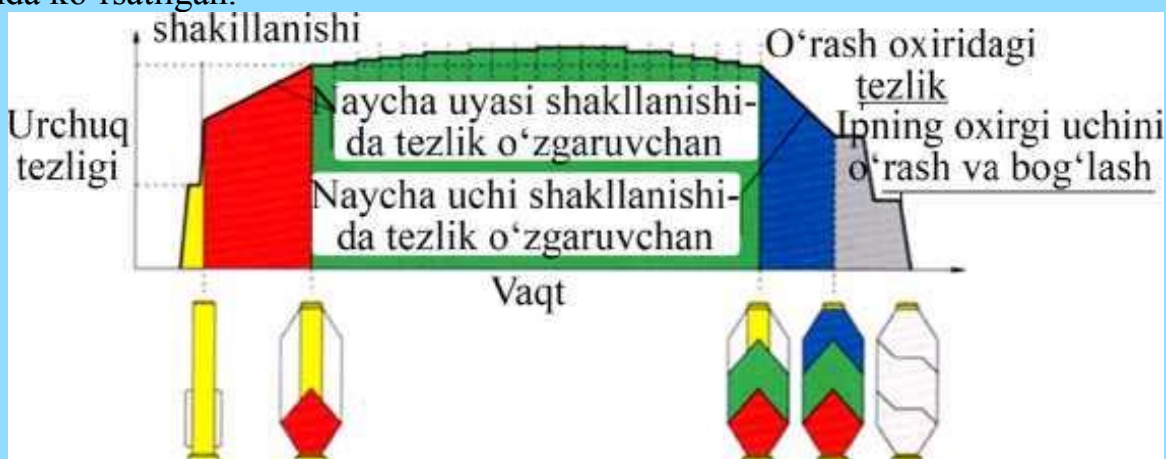
2.17-rasm. Halqali yigirish mashinasida naychaga ip o'ralishi sxemasi
