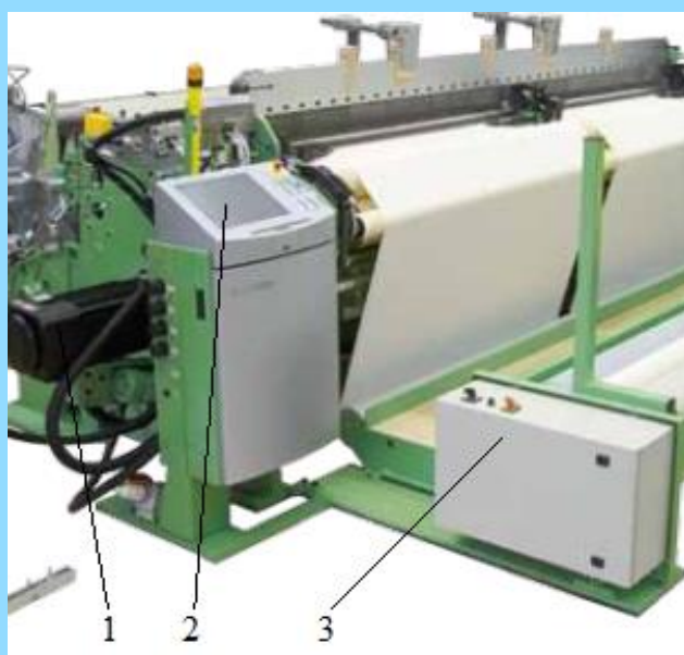
3.5-rasm. DORNIER to‘quv dastgoxi 1- DORNIER SyncroDrive motori, 2- boshqaruv paneli, 3-elektroquti.
