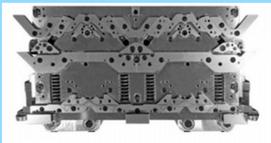
4.6-rasm. LongXing trikotaj mashinasining to`quv sistemasi
