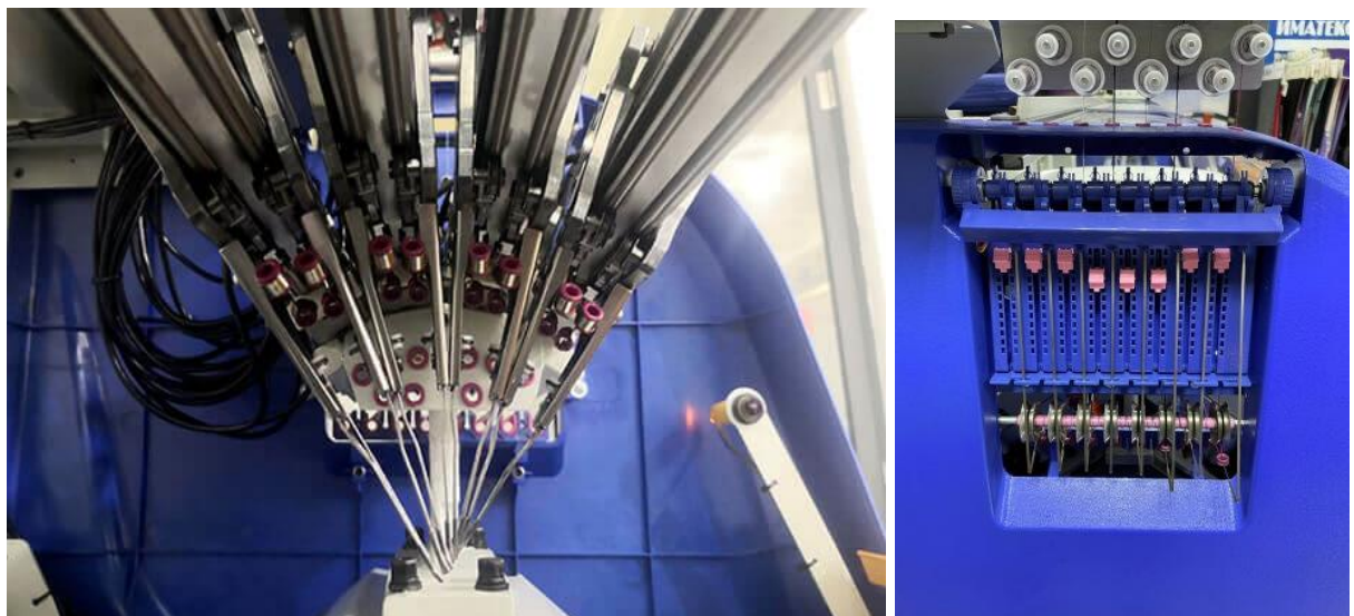
1.5-rasm. LongXing trikotaj mashinasining ip uzatish tizimi
