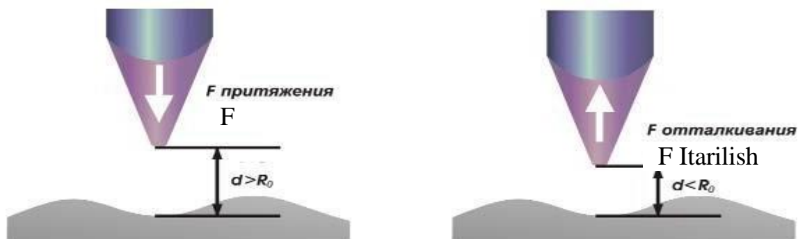
12-rasm. AKMning ishlash prinsipi
