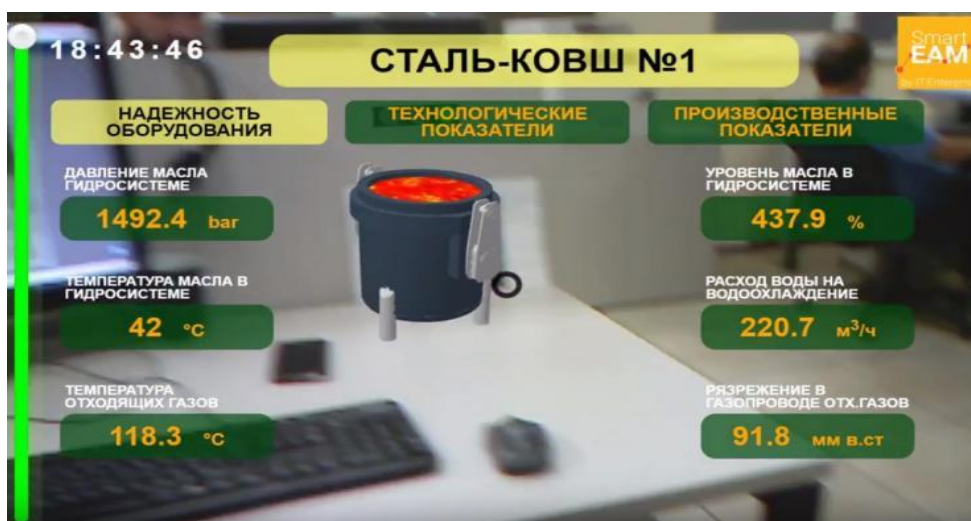
1.5-rasm. AR-ni INTERPIPE STEEL-da IT-Enterprise-ning SmartEAM yechimida qo‘llash misol
