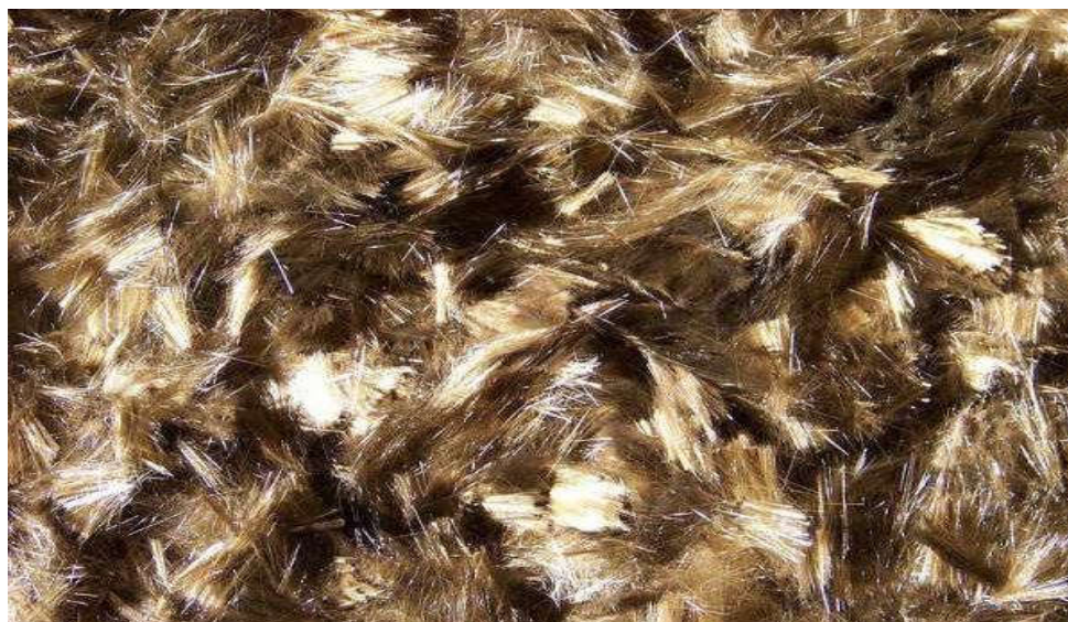
1-rasm. Bazalt tola va uni betonda qo‘llash.
