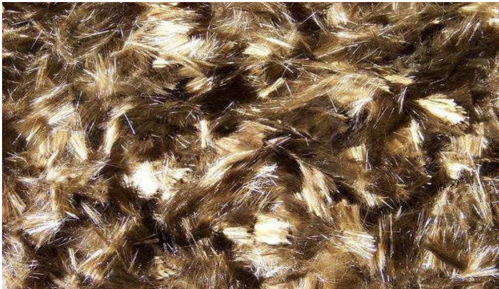
1-rasm. Bazalt tola va uni betonda qo'llash.
