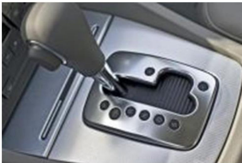
3.9-rasm. Tiptronik funksiyali AUQni boshqarish richagi
