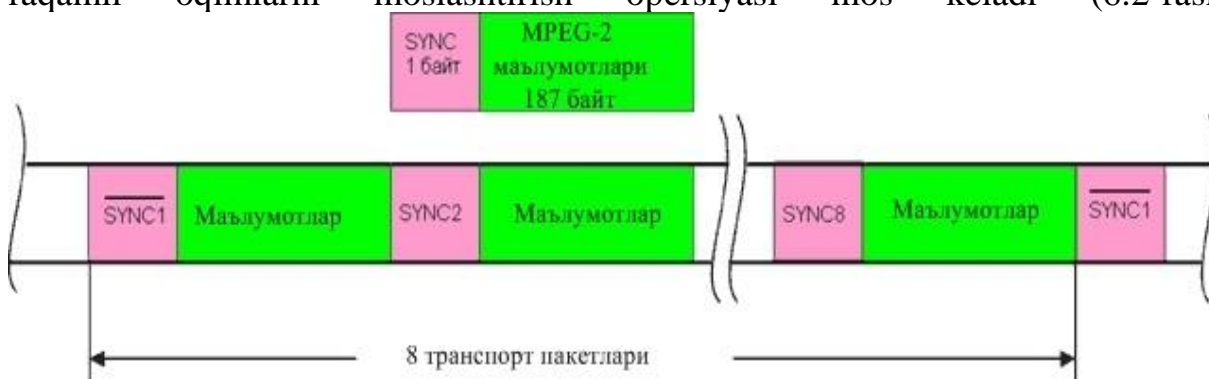
3.5-rasm. MPEG-2 ning transport paketlarining moslashuvi.
