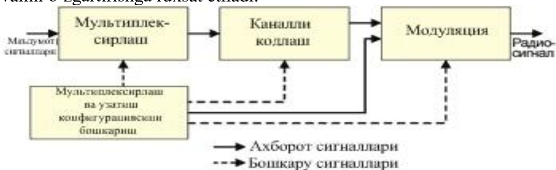
4.18 – rasm. ISDB – T tizimning uzatish chizmasi
