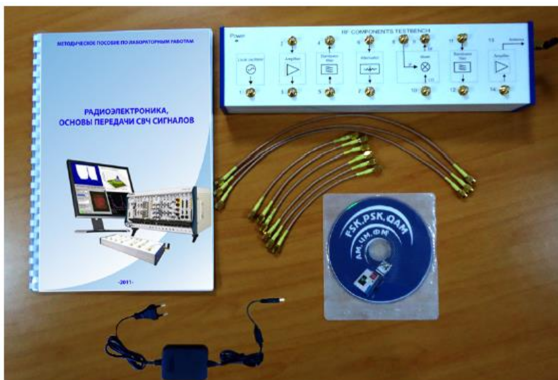
2-rasm. “RF Components Test bench” stendi elementlari.
