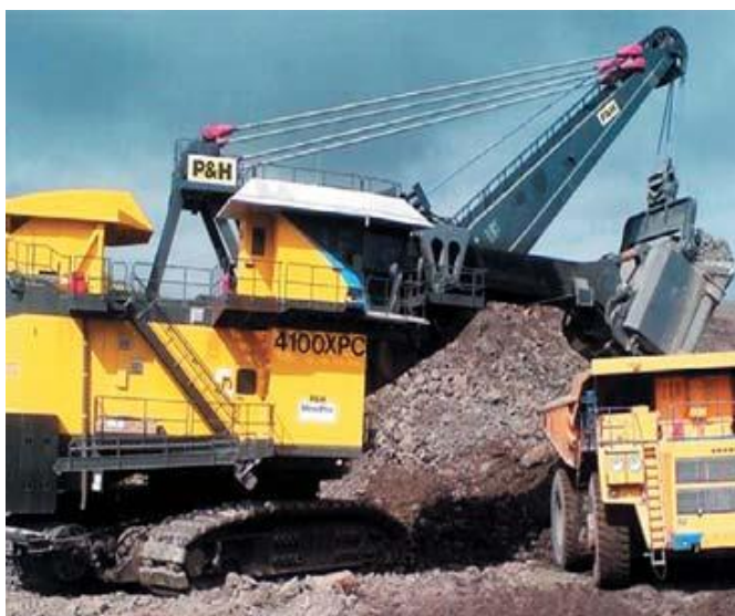
5-rasm. P&H kompanisining tishli reykali kuch berish tīmli 4100XRS eng katta karyer mexanik ekskavatori
