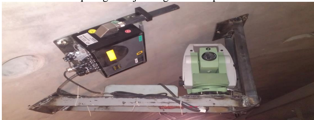
4-rasm: Yarim robotlashtirilgan lazerli taxeometr va siljuvchi radiomodem.
