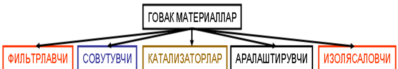
3.3-rasm. G'ovak materiallarining guruhlanishi.
