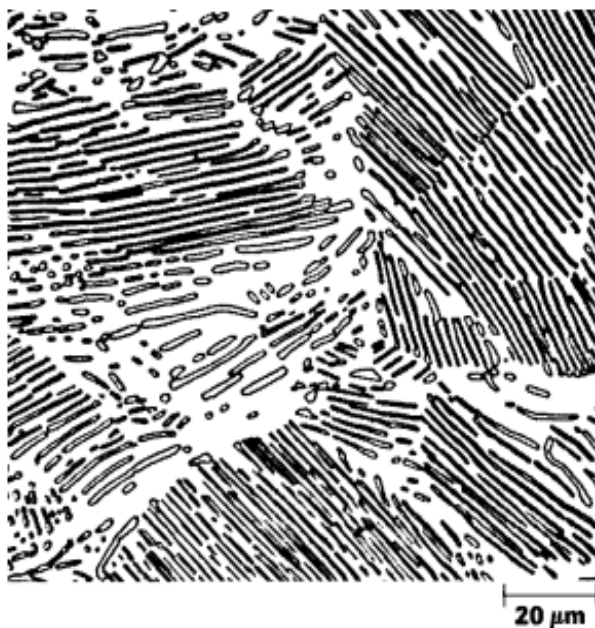
Figure 9.27 Photomicrograph of a eutectoid steel showing the pearlite microstructure consisting of alternating layers of \alpha ferrite (the light phase) and \text{Fe}_3\text{C} (thin layers most of which appear dark). 500 \times . (Reproduced with permission from Metals Handbook , 9th edition, Vol. 9, Metallography and Microstructures , American Society for Metals, Materials Park, OH, 1985.)
