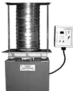
68-rasm. Zamonaviy KP-109.2 modeli sim g'alvir.
